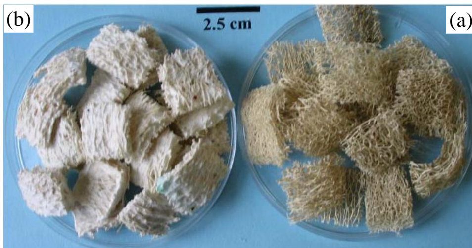
Fig. 2. Immobilization of P. chrysosporium within loofa sponge pieces: (a) loofa sponge pieces; (b) loofa sponge pieces covered with P. chrysosporium hyphal biomass.
