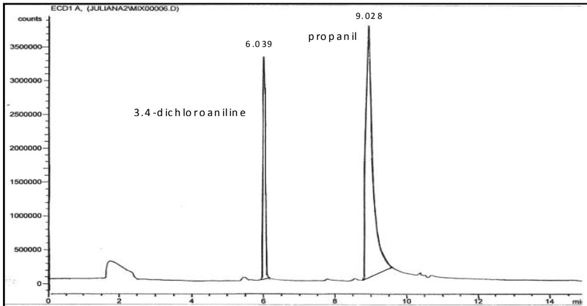
Fig. 2. Representative gas chromatography spectrum: analysis of propanil (>95% purity) and 3,4-dichloroaniline (>95% purity) dissolved in methanol.
