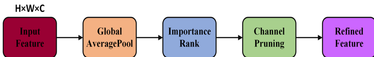
Fig. 8. Network architecture of the SF module.
