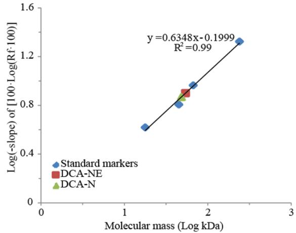
Fig. 5. Standard curve for molecular mass determination of DCA-NE and DCA-N. Logarithm of minus slope was plotted against logarithm of molecular mass of the standard markers. Logarithm of minus slope of DCA-NE, and DCA-N were used to calculate their molecular masses.
