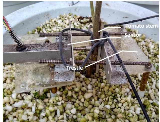
Fig. 1. The sensor used in diurnal measurement of the stem diameter in tomato.
