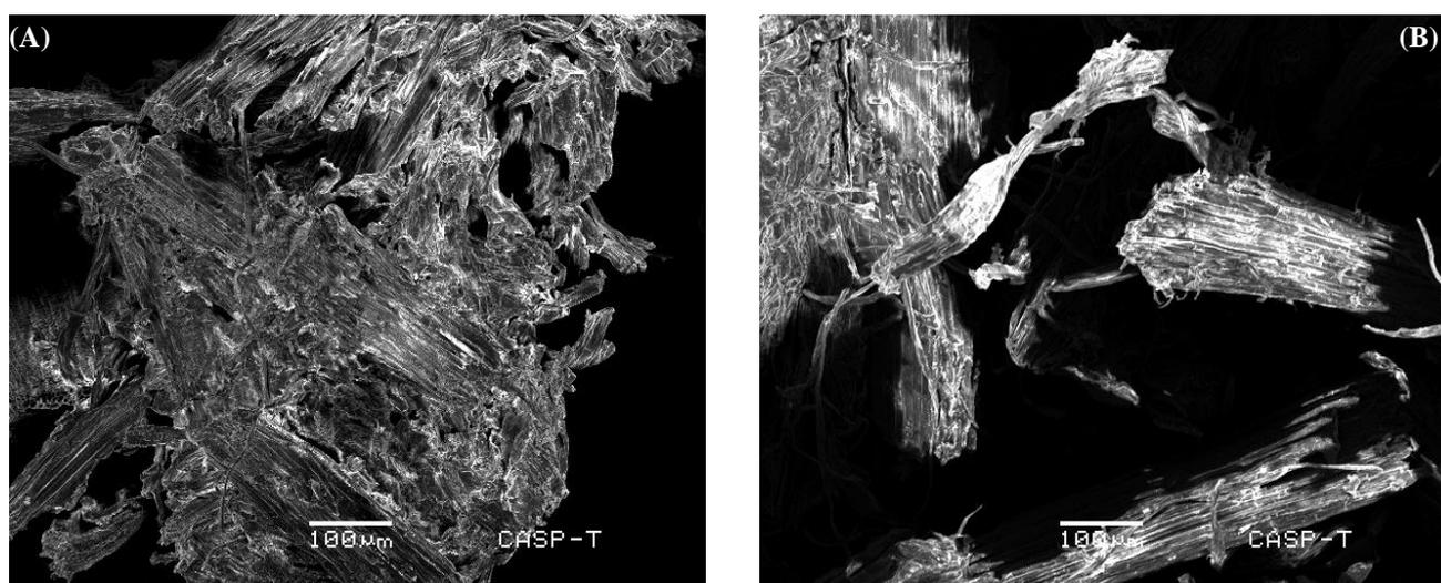
Fig. 5. Scanning electron micrograph of Sugarcane bagasse (A) before hydrolysis (b): after hydrolysis.
