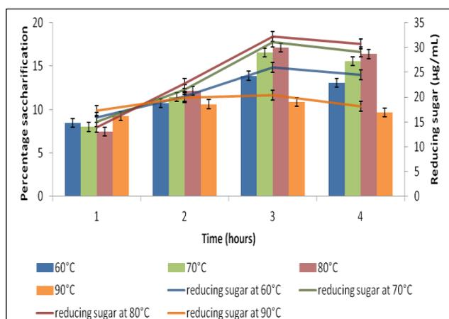
Fig. 3. Effect of different temperatures on the enzymatic saccharification of sugarcane bagasse A. Error bars indicate standard deviation ( $\pm$ SD) among three replicates.
