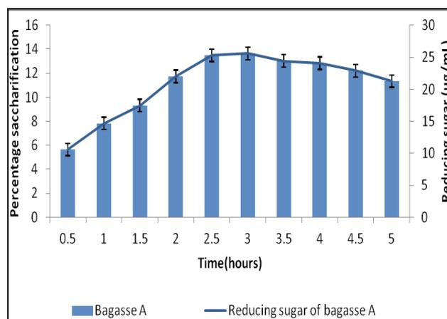
Fig. 2. Effect of incubation time on saccharification of Sugarcane Bagasse A. Error bars indicate standard deviation ( $\pm$ SD) among three replicates.
