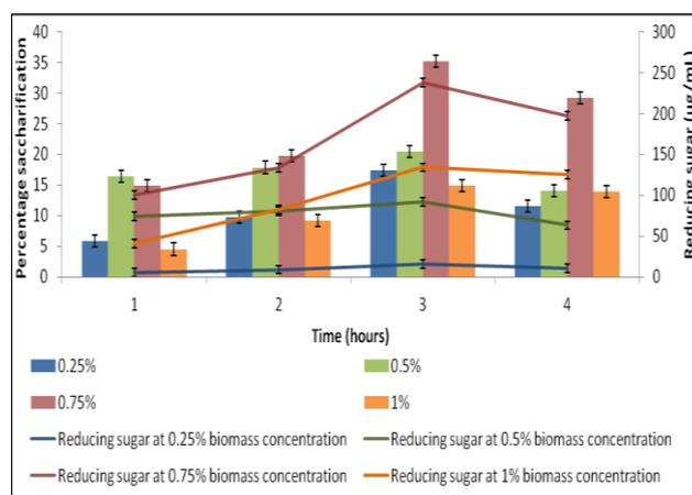
Fig. 4. Impact of various biomass concentrations on enzymatic hydrolysis of sugarcane bagasse. Error bars represent the significance of three determinants with a probability of  $\leq 0.05$ .
