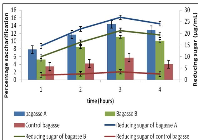
Fig. 1. Screening of pretreated sugarcane bagasse samples by enzymatic hydrolysis. Error bars indicate standard deviation ( $\pm$ SD) among three replicates.
