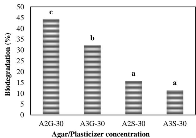
Fig. 4. Effect of different agar: plasticizer ratios on the biodegradation rates of agar films.
