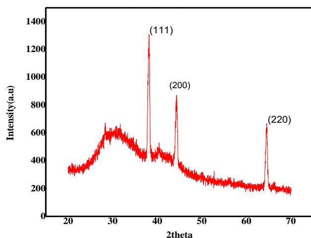
Fig. 5. XRD Spectrum indicate peaks for Au NPs.
