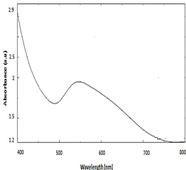
Fig. 3. UV- Visible spectrum show wavelength for Au NPs.
